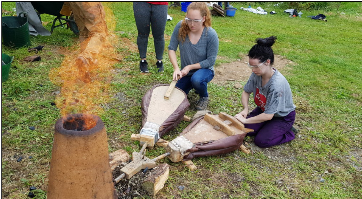
Students conducting an iron smelt at the Carrick Archaeological Site
